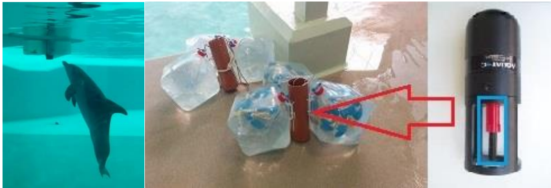
Figure 3. The test setups used in the present study. In figure 3a, a dolphin is echolocating towards the fish setup. In figure 3b, the control and the floats setup is shown. Arrow show the location of the PCL inside the orange plastic tube. Figure 3c show the PCL; the black rod inside the blue square is the hydrophone, which was pointed downward in the setups.
