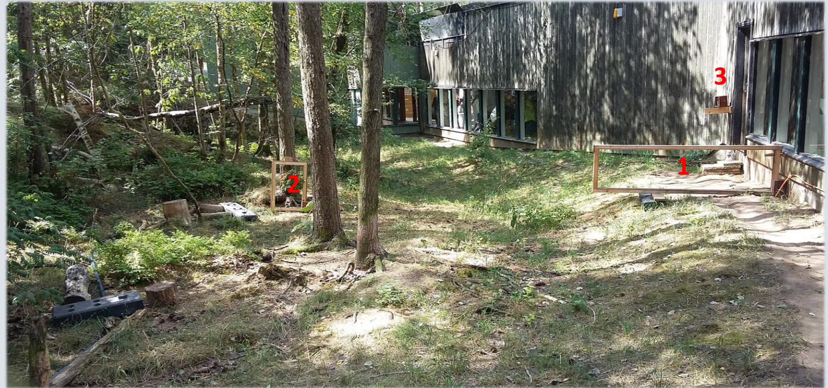
Automated monitoring. 1 : HDX PIT tag "pacing" antenna, 2 : Scent station with HDX PIT tag "scent" antenna and BLE tag, 3 : Reconyx Hyperfire wildlife camera.
