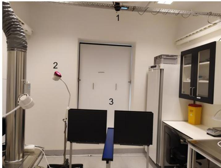
**Figure 2:** EPM set up. 1. Video camera; 2. Red light; 3. Maze.
